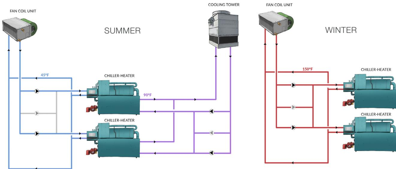
One of the secrets of implementing heat pumps is knowing that the lower the temperature they have to heat to, the more efficient they can be. The difference can be quite stark. In fact, a heat pump can consume twice as much electricity (and therefore \$\$\$) to produce the same amount of heat at 150F compared to 110F. The new thermal network substantially reduced the temperature, which opened the door for very efficient and cost-effective air-to-water heat pumps to be located on the roof.
